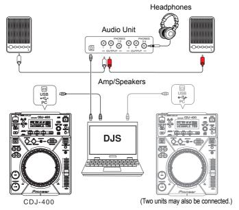
Configuration when using an External DJ mixer (Example of Connections) The DJS player A and player B audio is output to each audio output of your computer. Your computer needs to have two or more audio output systems.
