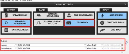
2) Even if "DDJ\_WeGO4 ASIO (ASIO)" or "DDJ-WeGO4" may be selected when you click "MICROPHONE" under "AUDIO SETTINGS" > "INPUT", DDJ-WeGO4 does not send the Mic sound input from the Mic terminal.
