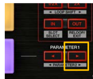
DDJ-SZ (Also for DDJ-SX, DDJ-SR, and DDJ-SP1, use the [PARAMETER (right)] button.)
