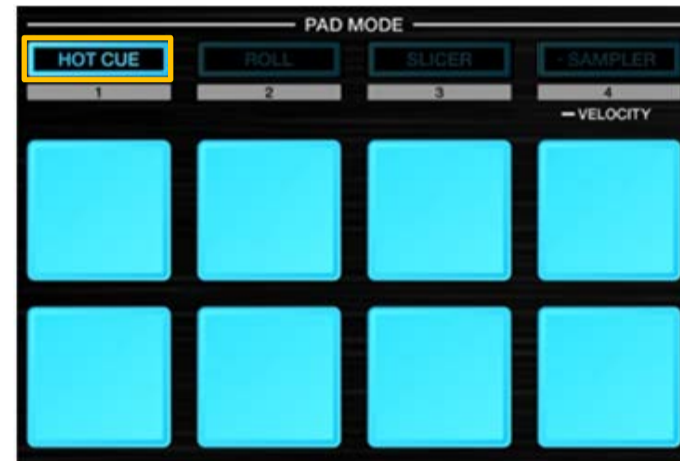
HOT CUE mode on DDJ-SX (For DDJ-SR and DDJ-SP1, use the [HOT CUE] mode button in the same location as in the above.)
