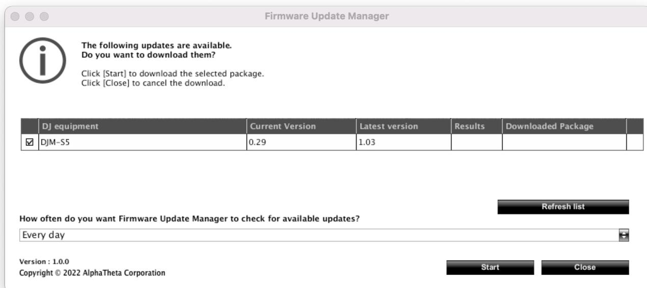
The window shows the current version installed on the connected device and the latest version available for download.
