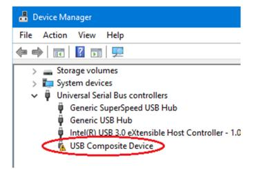
Disconnect the controller from the computer and uninstall the device driver on the controller.
