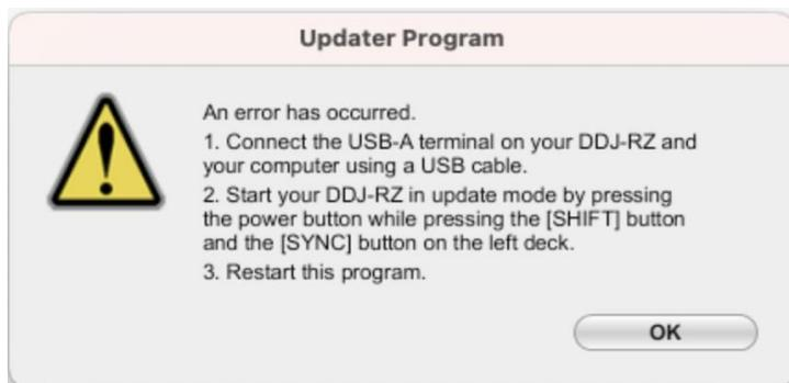
If the USB cable comes loose in the middle of the process or the unit turns off, redo the update process.
