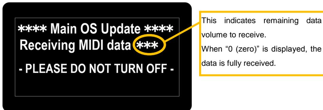
The number shown on the right of [Receiving MIDI Data] counts down as the data receives. When "0 (zero)" is displayed, the data is fully received.
