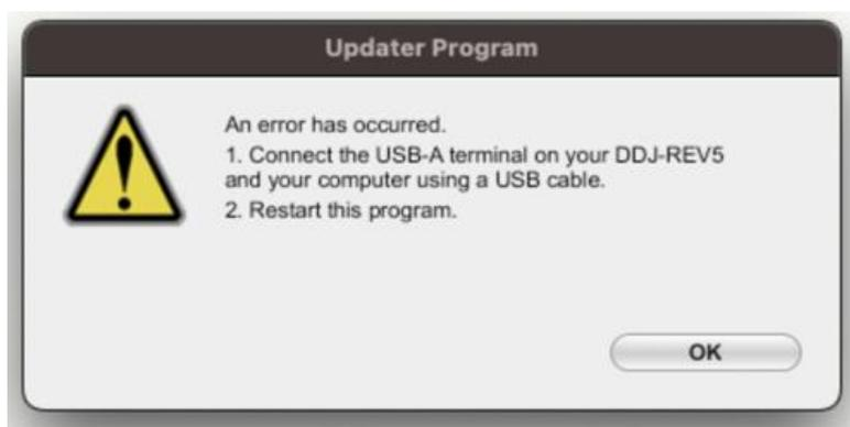
When the update is abnormally terminated, the DDJ-REV5 may launch in firmware update mode with the red at the top of the master level indicator flashing. In this case, please restart the update from “**D. Updating the firmware through your PC/Mac**” of the above updating procedures.
