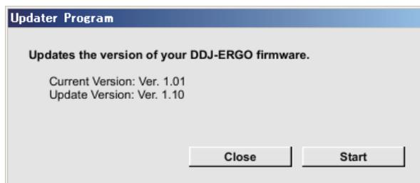
Updating starts. Do not turn off the power or disconnect the USB cable during updating.
